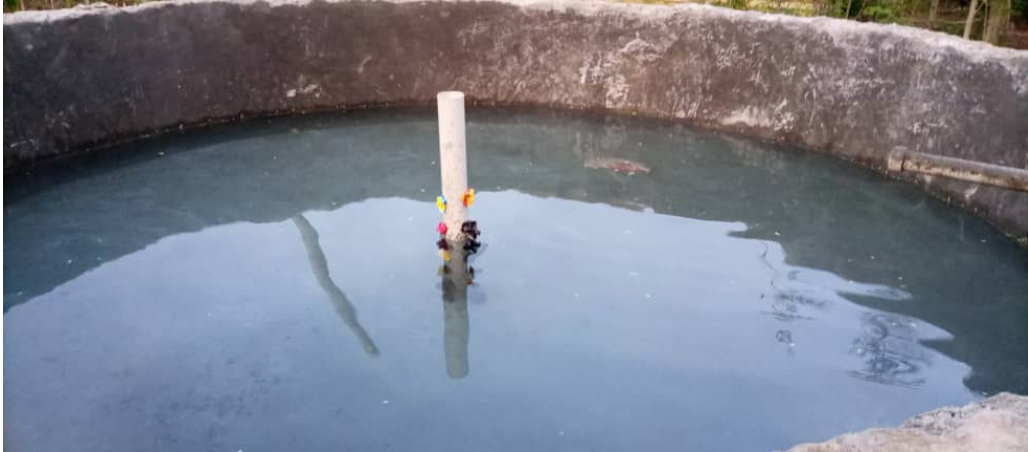
Testing of water retention capacity of tanks at Musukwe fishfish
